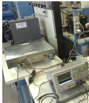
The LAB bench with the AC/DC for grid connection
