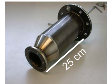
vertical evaporator (25 kW), ISE 2007
