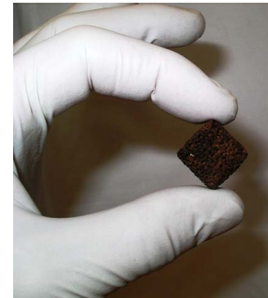
CPOX catalyst for 125 W SOFC generator
