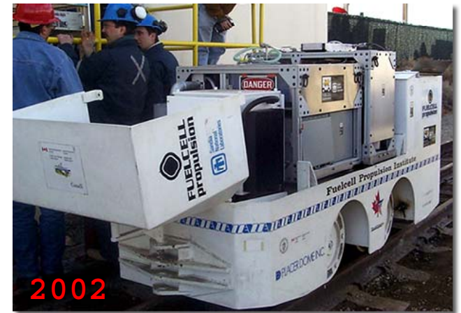
Fuelcell mine locomotive, a non-hybrid
